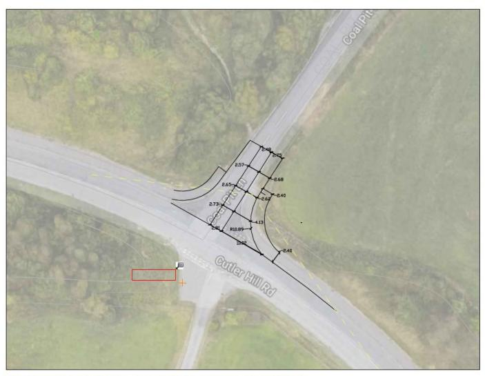
INTRODUCTION OF ADDITIONAL LANE ON APPROACH AT COAL PIT LANE AND RECONFIGURATION OF CARRIAGEWAY, FOOTWAY AND ROAD MARKINGS.
